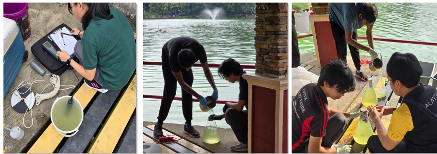
Figure 3. The involvement of citizen scientists in their on-site activities at Taman Aman Lake, as seen from left to right, perform water quality testing using a multiparameter water quality meter, collecting water samples and labelling water samples.
